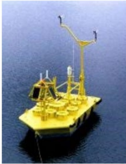
Figure 2-5: 6-Meter Boat-Shaped Hull Buoy Source: National Data Buoy Center 2012
