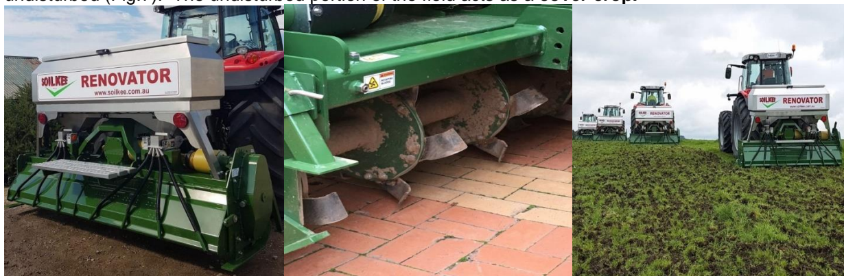
Figure 5. The Soil Kee renovator/ Planting system used in Australia to facilitate carbon sequestration
